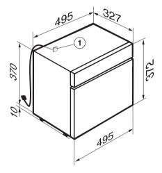
1) Inlet for mains connection cable to the appliance
